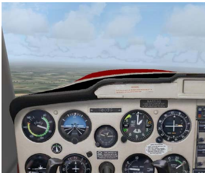
Figure 1- Cruise Configuration . Note 1000 Ft and North. RPM set to 2200RPM- (or equivalent cruise power for aircraft).
