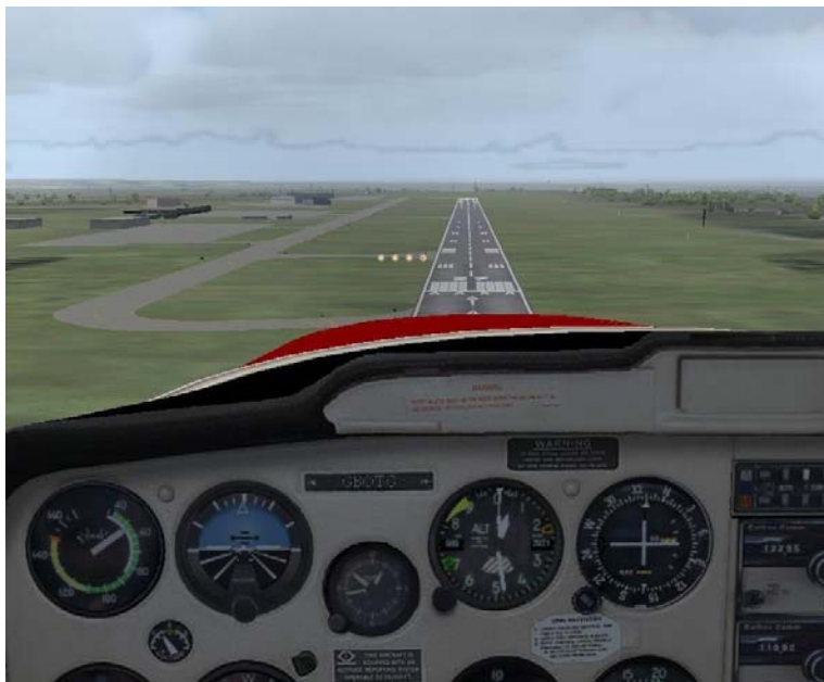
Figure 4- Keep the touchdown point constant in the window using power adjustments. Don't let speed fall-off completely however! (Spot the error- speed is not appropriate in this picture!)
